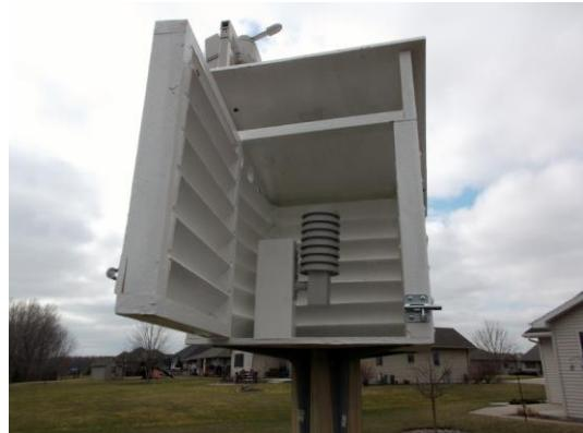
What does a retired meteorologist do when the cold winds blow and all the lakes and streams are covered in ice? He builds a thermoscreen, of course. Having long since tired of bum readings caused by wrong exposure, I decided it was time to do what the Navy Weather Service did decades ago – house the sensors in a thermoscreen.
