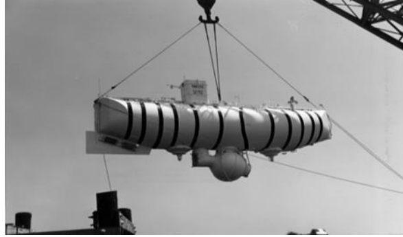
Bathyscaphe Trieste entering the water in April 1959. The Observation gondola that Walsh and Piccard occupied during the dive can be seen center bottom. National Archives Photo
