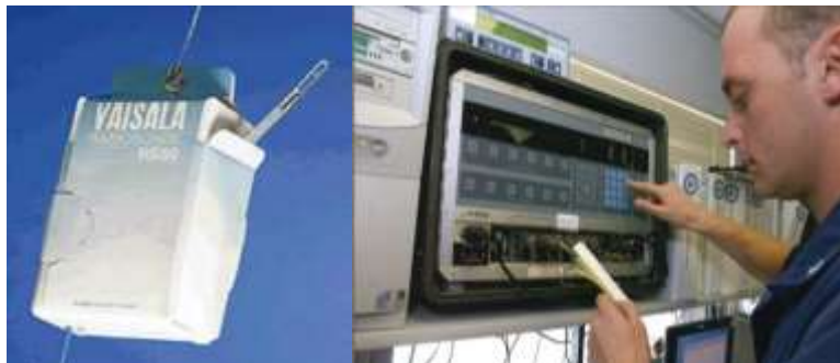
RS80 Radiosonde. AG3 Giacometti programming information into the AN/UMQ-12 MRS Receiver before balloon launch. (U.S. Air Force photo by Staff Sgt. Jocelyn Rich taken in the British Indian Ocean Territory (June 21, 2005))
